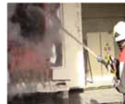
Hose Stream testing
