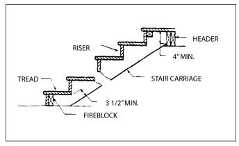
Fireblocking is used between stair stringers at the top or bottom of the run.
