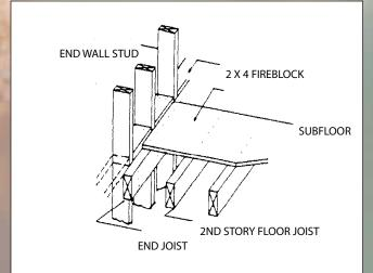
Fireblocking can be used to block off a stud space in a wall.
