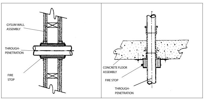
Examples of through-penetrations in fire resistance-rated assemblies that have been firestopped.
